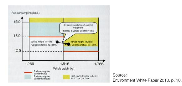
Figure 4 Transitions of vehicle weights and fuel consumption standard values
