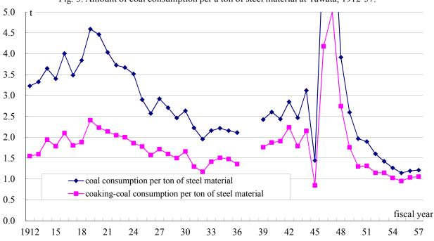
Fig. 3. Amount of coal consumption per a ton of steel material at Yawata, 1912-57.
