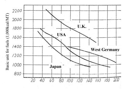
Capacity of an open hearth furnace (MT)
